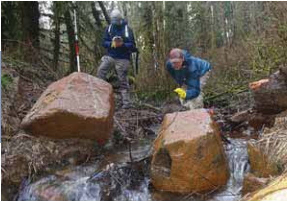
Technicians conducting a stream crossing pebble count as part of a post-decommissioning inventory.
