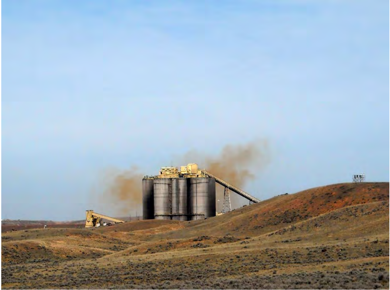
Orange nitrogen dioxide cloud produced by blasting at the Jacobs Ranch Mine on April 11, 2010 in the Powder River Basin, Campbell County, Wyoming. 76
